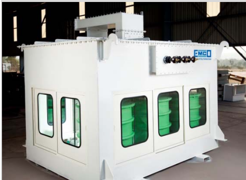
High Temperature Superconductor (HTS) Transformer
